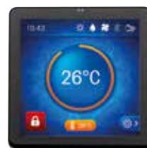
Lockable TFT screen to prevent tampering
